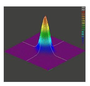
Ti:sapphire Laser(10mJ @ 1kHz pumping @ 527nm by DS20-527)
