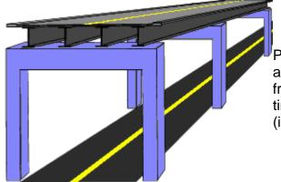
Pi shaped rigid frame structures are used frequently as the piers and supports for inner city highways. The frame supports the raised highway and at the same time allows traffic to run directly under the bridge (illustration #2.)
