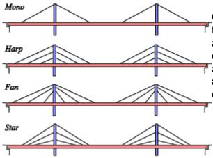
Cable arrangements also vary greatly. Some typical varieties are mono, harp, fan, and star arrangements (illustration #4.) In some cases, only the cables on one side of the tower are attached to the girder, the other side being anchored to a foundation or other counterweight.
