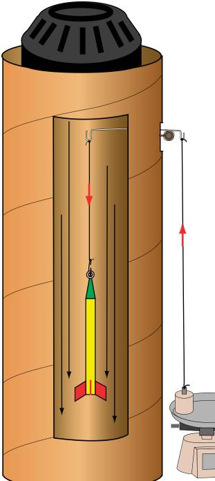
The cardboard cement form is available from large hardware stores. It generally comes in 8" and 12" diameters. You will need a strong fan to power the tunnel. The 12-inch tube provides students with more flexibility in their rocket designs. It permits fin spans of nearly 12 inches.
