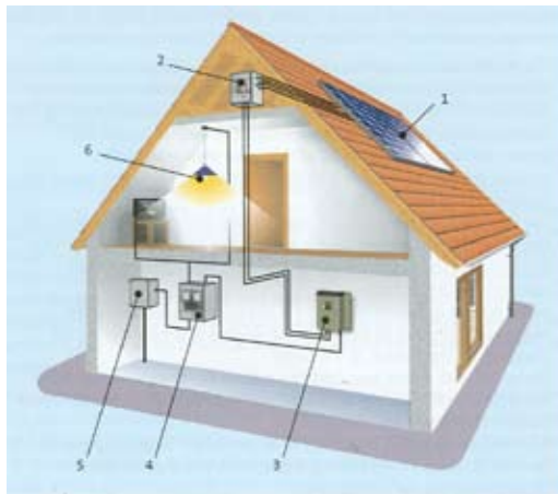
Figure 2.8 Schematic of a typical grid-connected PV system
