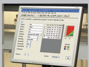
ChromQuest's instrument control provides an easy and uniform way to control all LCs and GCs. Software controls extend to the instrument autosampler, detector, temperature controls, injection controls, and pump. The software display of the new Accela High Speed LC pump with its unique quarternary pump controls is shown.
