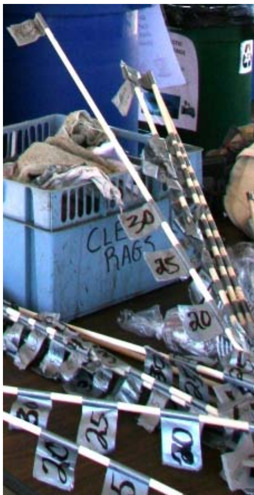
Figure 3. Picture of volume measuring dowels. Examples of measuring dowels used to calculate the volume of materials.
