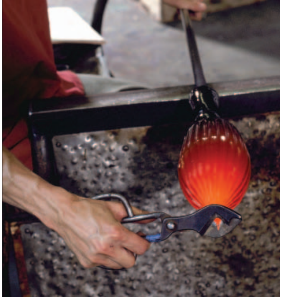
A glassblower uses heavy shears to cut a piece of molten glass.
