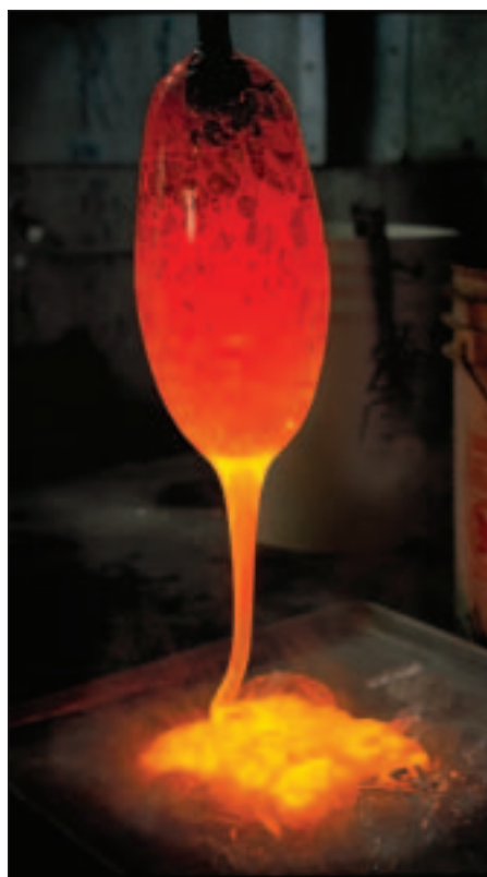
Molten glass flows from a gather collected on the end of a blowpipe.
