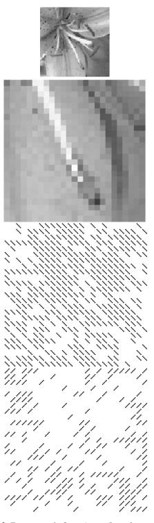
**Figure 2:** Top: a part of a flower image. Second: a magnified view of the bottom stamen. Third: the pixel level data dependent triangulation of the stamen (NW-SE direction) Bottom: NE-SW direction
