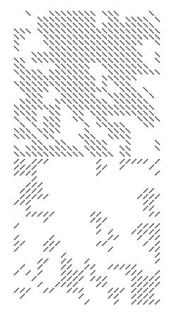
**Figure 4:** *The triangulation mesh of the extended method. Top: NW-SE direction. Bottom: NE-SW direction*
