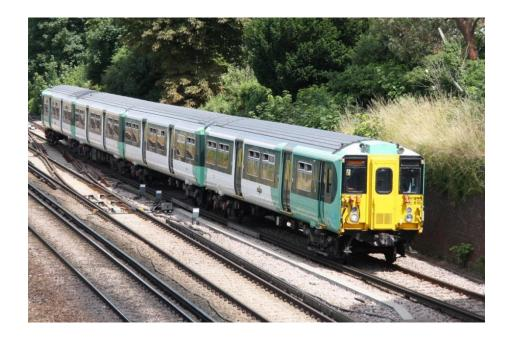
The Class 455 is an inner-suburban EMU, designed for the southern DC network. Its high capacity interior is laid out in 3+2 seating configuration. On-train systems data is automatically downloaded into the Train Automatic Performance Analysis System (TAPAS) which drives condition-based maintenance. Minimal work is required to achieve targeted PRM TSI accessibility compliance.
