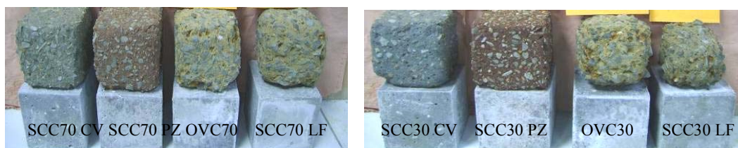
Figure 9. Deterioration of specimens after 12 weeks of immersion in 5% HCl solution
