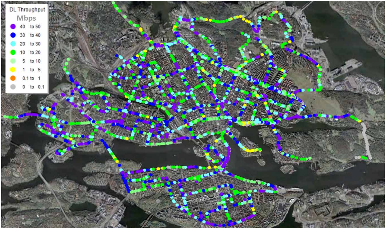
Figure 74: Drive Test of Commercial European LTE Network (10+10 MHz) 161
