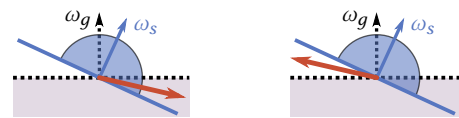
Fig. 3. Problems caused by normal mapping. With a naive approach, light can leak through the surface when evaluating the BRDF with respect to the shading normal (left). Furthermore, the BRDF is undefined for directions below the tilted hemisphere defined by the shading normal (right).
