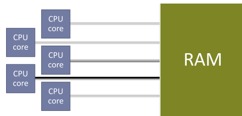
Figure 2: An idealized multiprocessor where cores take sequential turns accessing a single shared set of memory.
