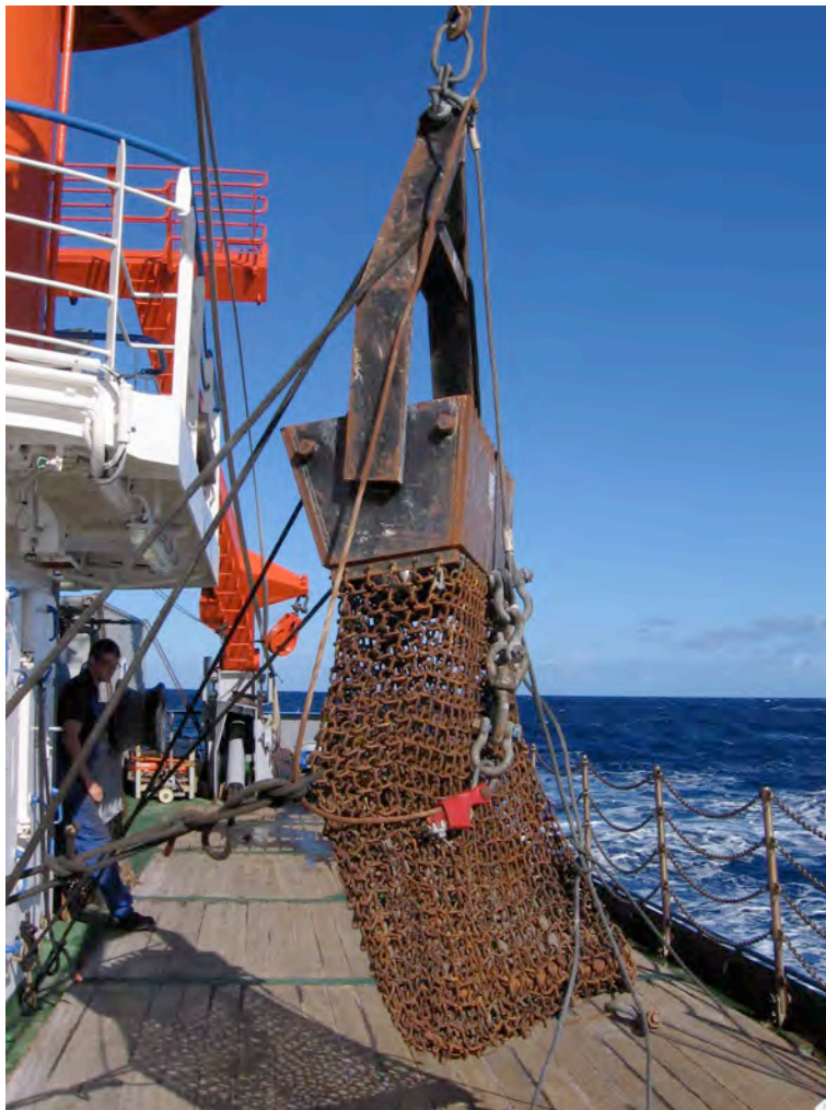
Figure 2. A chain sack dredge of the Department of Magmatic and Hydrothermal Systems at IFM-GEOMAR on the port side deck of the German research vessel Poseidon. Photo: POS 379/1 Scientific Party.
