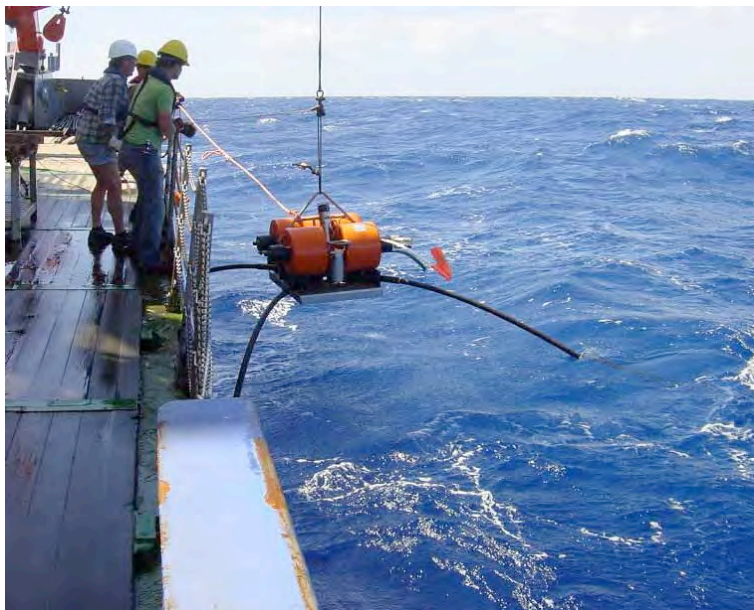
Figure 3. A MT-Lobster station (designed at the IFM-GEOMAR in Kiel) is deployed on Poseidon cruise POS-379/2.
