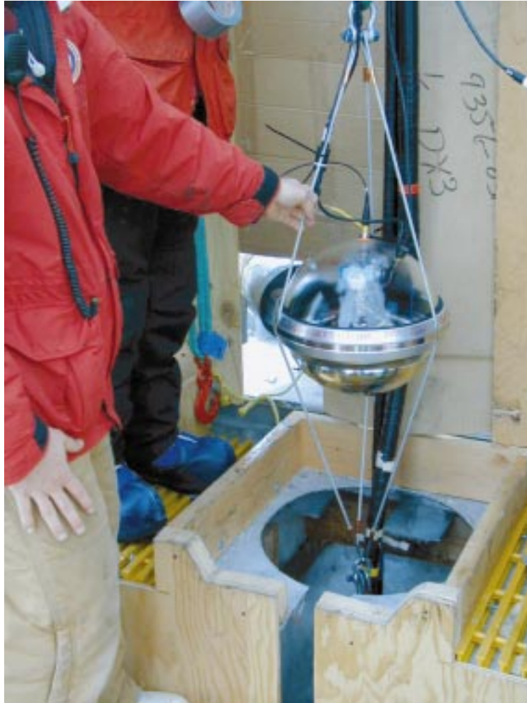
Figure 78: An OM ready to be lowered into the drill hole.
