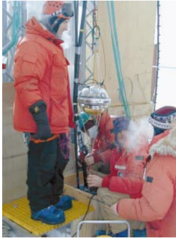
Figure 77: Installation of an OM.
