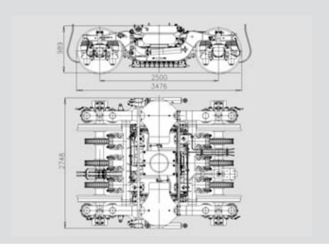
For damping of lateral and vertical movements, hydraulic dampers are installed.
