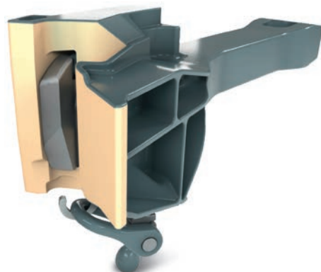
Voith Standard SA3 Coupler Head featuring Mixed Coupler Device
