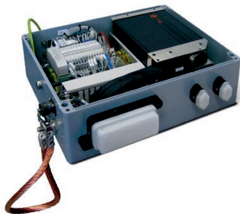
Coupler and Front Hatch Control Unit, Cover Removed
