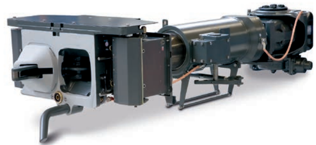
Type 35 Automatic Scharfenberg Coupler Featuring Electric Heads and Centring Device
