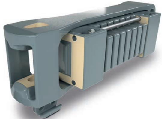
Draft Gear with Yoke with Reversible Energy Absorption
