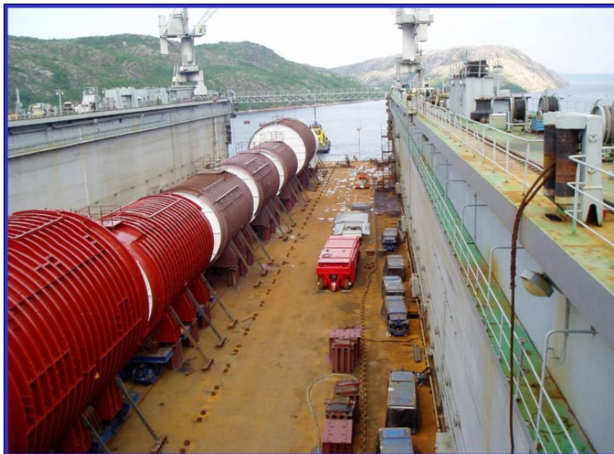
Figure 5. Transportation of reactor compartments in the floating dock
