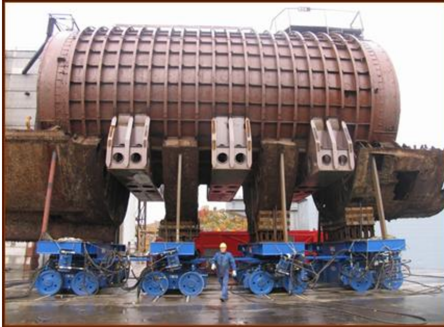
Figure 4. Testing of German docking-block transport system at Nerpa shipyard
