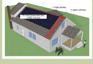
A 3-foot setback from all roof edges shall be provided for roof mounted solar panels to ensure that firefighters may access the roof in a quick and safe manner.
