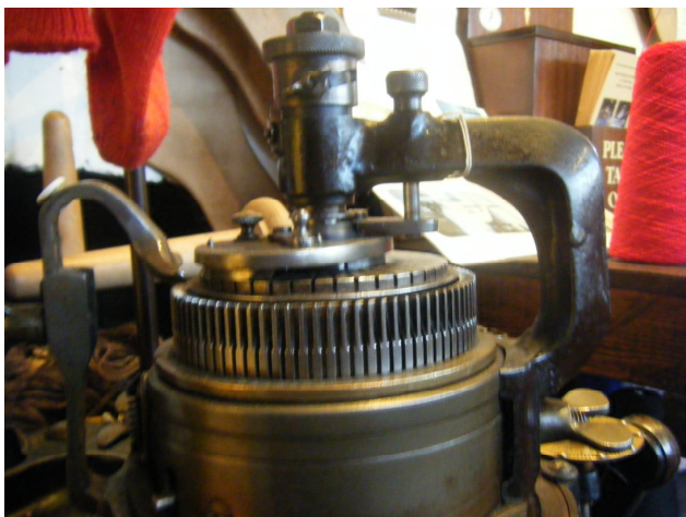
← A Harrison table mounted machine with top ribber in position
