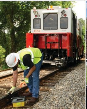
1 Using Rail Flaw Detectors to Test for Rail Defects
