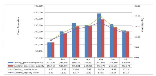
Figure 6. Comparison Graph of Juam Dam Floating-overland Power Generation
