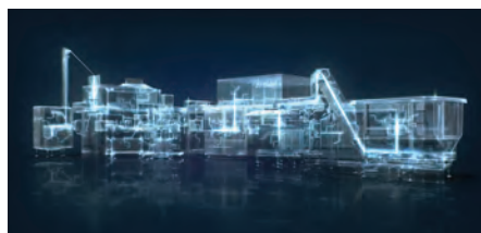
Sidel Super Combi, integrating five process steps – preform feeder, blower, labeller, filler/capper and cap feeder - into an all-in-one smart system, was awarded the 'Best Manufacturing or Processing Innovation' at Drinktec.
