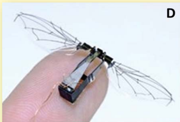
D. Harvard researchers are pushing the technology on an even smaller scale with their RoboBees project (above), which emulates a colony of honeybees containing insect-sized flapping-wing robotic platforms. These biomimetic platforms have the added advantage of stealth. 9
