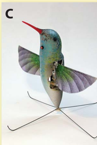
C. Scientists also are studying the way birds and insects fly to better understand aerodynamics and low-noise systems. The Nano Hummingbird (above) demonstrated controlled, precision hovering and fast-forward flight of a two-wing, flapping-wing aircraft that carries its own energy source and uses only its wings for propulsion and control. 8
