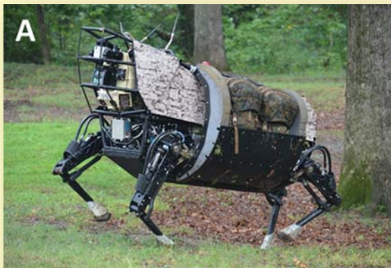
A. The Defense Advanced Research Projects Agency (DARPA)-funded BigDog robot uses four animal-like legs to traverse terrain too rough or slippery for conventional vehicles. It is also capable of recovering its “balance” if it slips. The current iteration of the program, the Legged Squad Support System (LS3) (above) seeks to demonstrate that a highly mobile, semiautonomous legged robot can carry 400 lbs. of load through rugged terrain. 6
