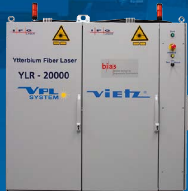
20 kW fiber laser, made by IPG Laser GmbH, Burbach
