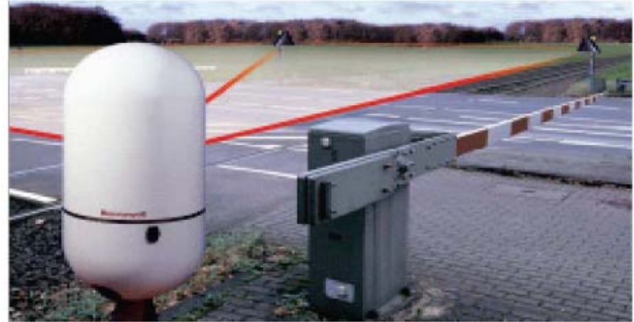
Figure 6.11 – MCB-OD Radar (top), Lidar (bottom left) and the area of obstacle detection provided by both
