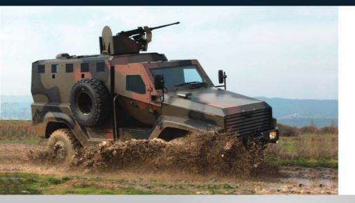
KAYA is especially designed and developed as a Mine Resistant Troop Carrier. Based on Daimler Chrysler UNIMOG 5000 chassis; KAYA provides excellent mine and ballistic protection along with high cross country capability and crew comfort in all terrain conditions.
