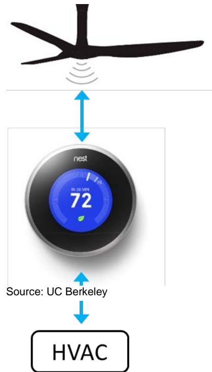
Figure 24: Auto Controlled, Learning Ceiling Fans and Thermostats
