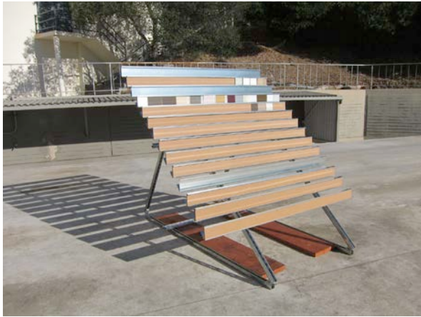
Figure 12: Exposure Rack for Cool Wall Products Constructed Onsite at LBNL
