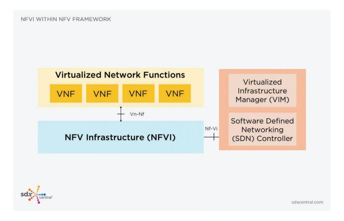
The NFVI layer primarily interacts with two other NFV framework components: VNFs and Virtualized Infrastructure Manager (VIM). The VIM, on the other hand, is responsible for provisioning and managing the virtual infrastructure. This means that the VNF to NFVI interface (Vn-Nf) constitutes a datapath through which network traffic traverses, while the NFV to VIM interface (Nf-Vi) constitutes a control-path that is used solely for management but not for any network traffic.
