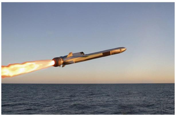
The design of the NSM emphasises the penetration of ship defences through a combination of low observability, onboard intelligence, and endgame kinematics. (Kongsberg)
