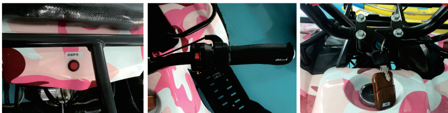
启动开关/Start switch 方向开关/Directional switch 电门锁/Electric door lock
