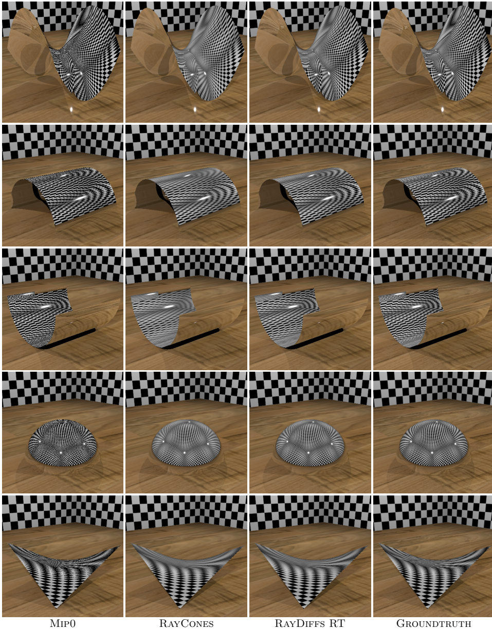
Figure 11: Comparison of textured reflections for different types of surfaces using different techniques. The GROUNDTRUTH images were rendered using 1,024 samples per pixel and by accessing mipmap level 0 for all texturing. For RAYCONES, we used the sign function in Equation 33.
