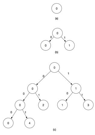
Fig. 2: Example of a sharding tree structure
