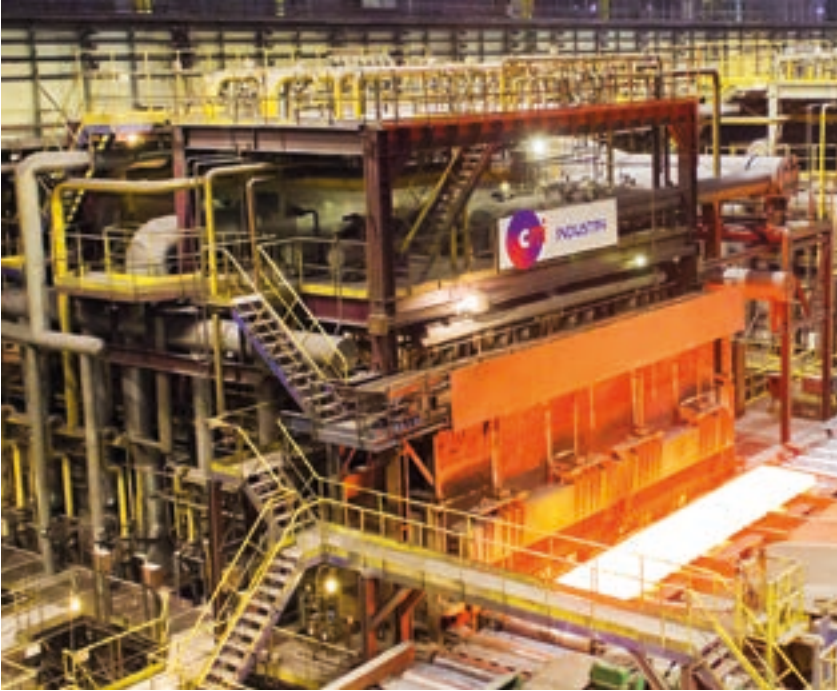
▲ The double regenerative burner technology developed and patented by CMI Industry drastically reduces the operating costs of slab furnaces and revolutionizes the cost of hot-rolled coil.
