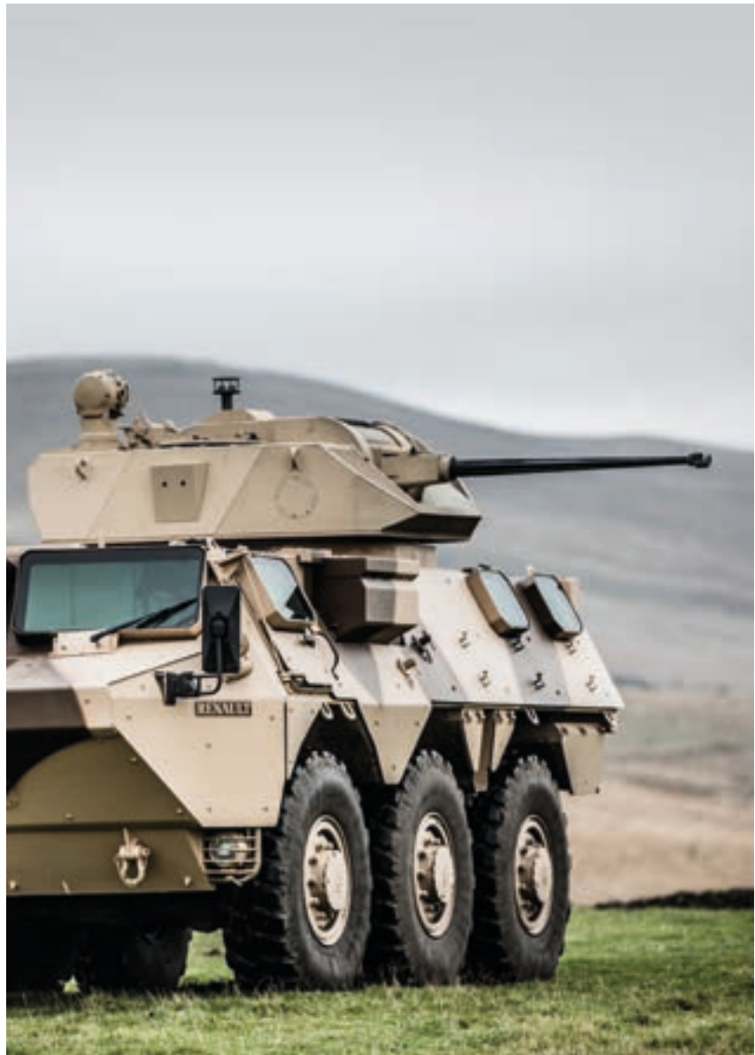
▲ Cockerill gun-turret systems cover the range of calibers from 20 to 120 mm. Here, the remotely operated Cockerill CPWS station equipped with a 25 mm gun.
