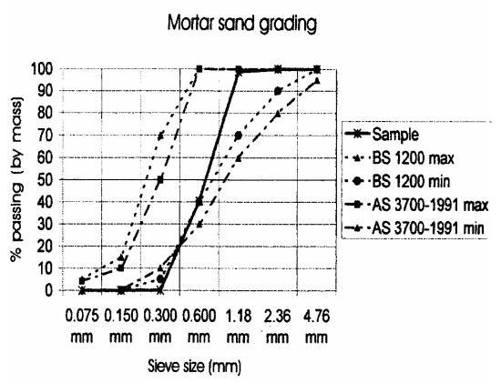
Figure 1 - Sand grading for permeable mortar compared to BS 1200 and AS 3700-991 recommendations (Jordan 2004) (Note that a mortar for successful carbonation barely falls within the ranges specified by the standards. A more suitable mortar would most likely fall without.)
