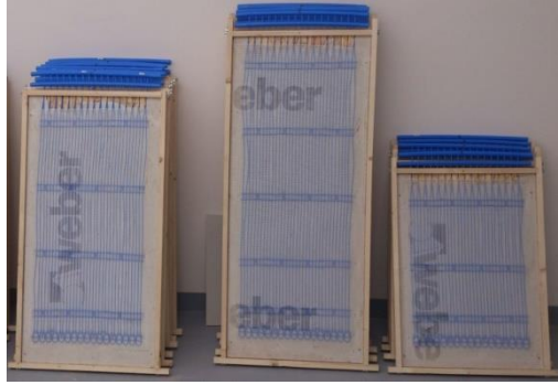
Figure 3.33: Base plates with attached plastic tubes
