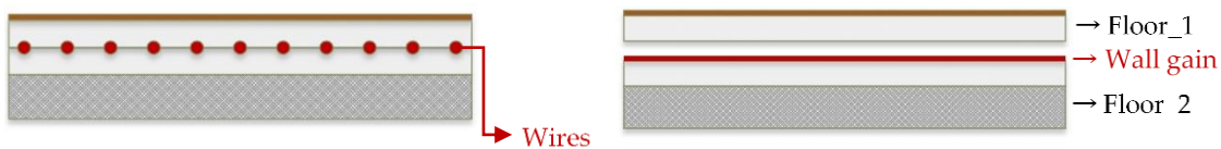
Figure 3.9: Conventional configuration of an EHF (electrically heated floor) (left) and configuration of the floor in TRNSYS with the added fictitious zone and the wall gain (right)
