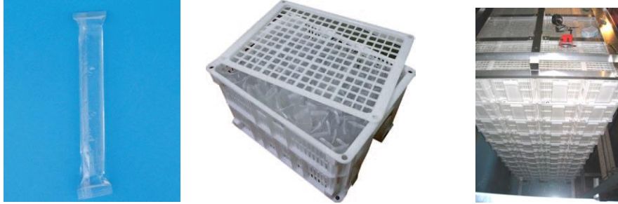
Figure 3.27: Latent heat thermal storage material package or gel pack (left), plastic case filled with gel packs (middle), and typical installation of the plastic cases into the isolated tank (right)
