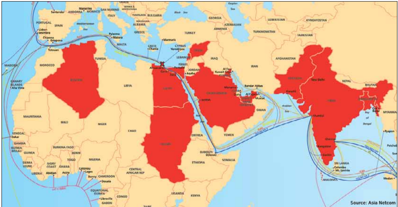
Figure 4. Multiple cuts in two undersea intercontinental cables. The countries in red were most affected by the cuts (red x above Egypt), which occurred on January 30, 2008. The two cables accounted for 76 percent of the transmission capacity among Europe, the Middle East, North Africa, and India. Image courtesy of Earl Zmijewski, Renesys; www.renesity.com/blog/2008/01/mediterranean_cable_break.shtml .
