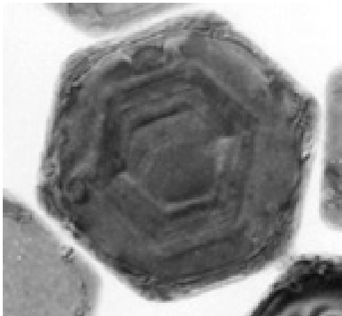
Photo 10 Multi structured sigma crystal grain.
