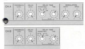
The stereo ping-pong effect in example 4 is achieved by setting the delay time on Channel A to exactly half the time of Channel B. The effect is like having the Channel A delay time setting with 2 repeats; one on the left followed by one on the right. Adding feedback to either A or B can cause lingering effect in which the stereo is less obvious than the first 2 repeats.
