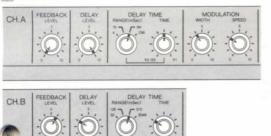
In example 3 Channels A and B operate very differently, A doing chorus while B does delay. When one instrument is used and footswitches are hooked up to both units, either effect is available and both can be combined along with the dry sound, for a total of 4 "presets" easily footswitched live. In the second patching example the two effects can be used simultaneously on different instruments.
