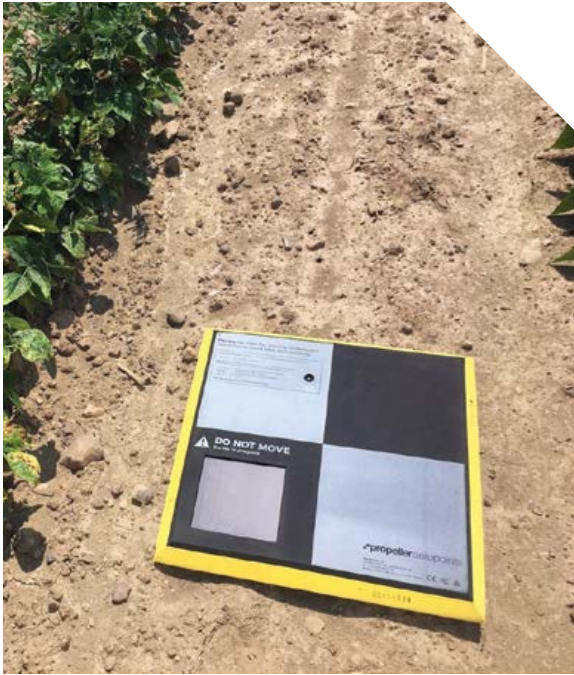
GPS-embedded reference targets placed in each scene enable precise geo-location and registration of image data.
