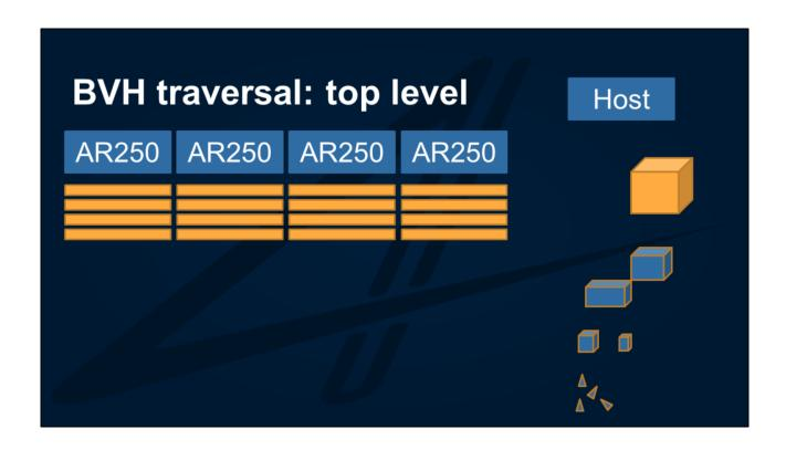
In more detail: All rays on the AR250s (orange) are intersected with top level of the BVH (orange).
