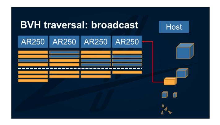
Since the AR250s report hits, geometry for the next level of the BVH is broadcast from the host to the AR250s.
