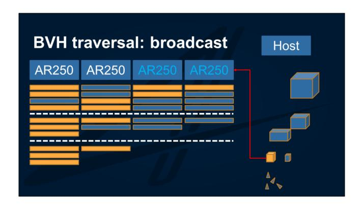
Two of the AR250s are still active, so the next level of the BVH is broadcast. If none of the AR250s were active, BVH traversal would stop at this point, and we would move on to the next unvisited node.
