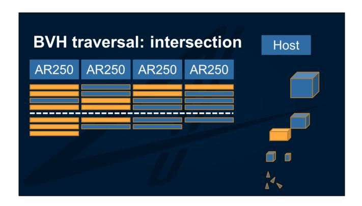
The live set of rays is intersected against the new geometry – on this occasion, only the first two AR250s contain rays which hit.
