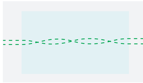
FIGURE 118 In certain materials, light beams can spiral around each other.
