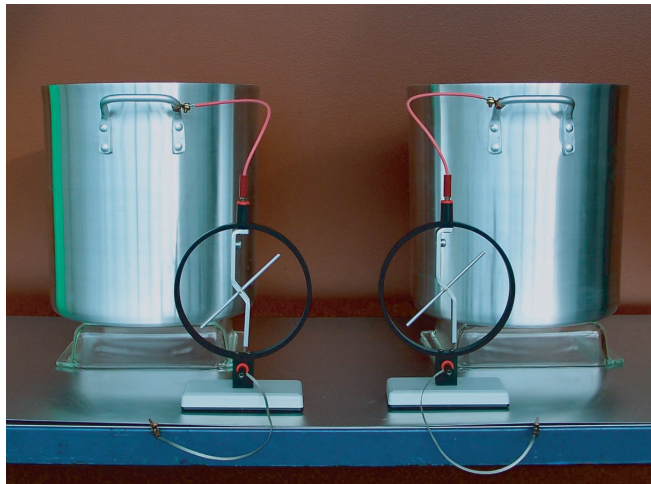
FIGURE 8 A simple set-up to confirm electric charge conservation: if rubbed fur is moved from the first pot to the second, the charge taken away from the first pot is transferred to the second, as shown by the two electrometers (© Wolfgang Rueckner).
