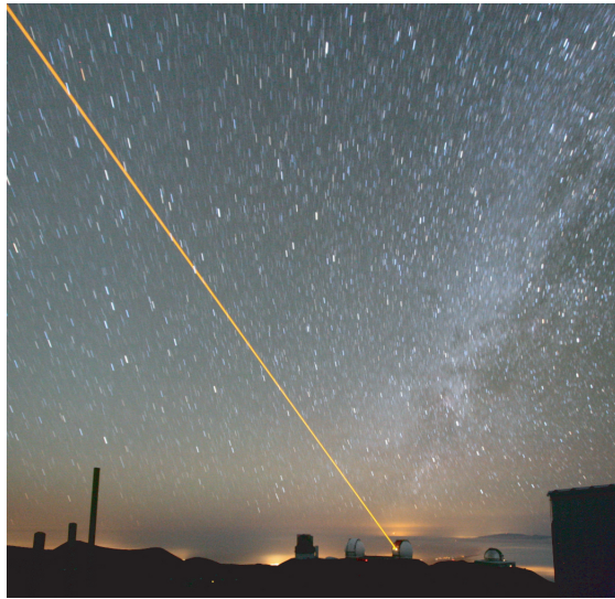
FIGURE 100 Light usually travels in a straight line. In the figure, a sodium frequency laser beam is used as laser guide star to provide a signal for adaptive optics in large telescopes. The laser illuminates a layer of sodium found in the atmosphere at around 90 km of altitude, thus providing an artificial star. The artificial star is used to improve the image quality of the telescope through adaptive optics. In the photograph, the images of the real stars are blurred because of the long exposure time of 3 min (photo by Paul Hirst).
