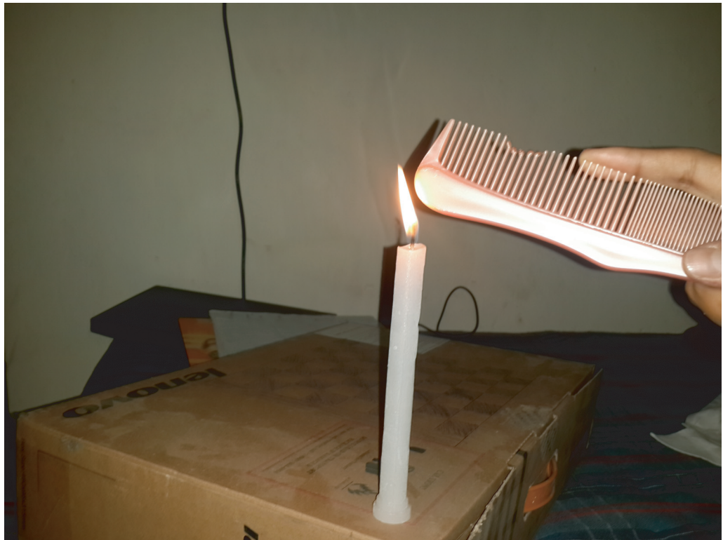
FIGURE 185 The way a flame reacts to a rubbed comb (© Shubham Das and Rakesh Kumar).
