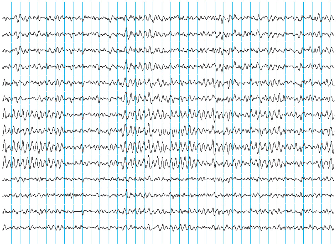
FIGURE 174 A modern electroencephalogram, taken at a number of positions at the head. The measured voltages are around 0.1 mV (© Wikimedia).
