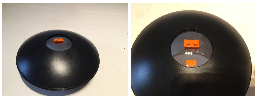
FIGURE 128 A floating Lego brick displayed by two stacked parabolic mirrors, the upper one with a hole. The right picture shows both the brick lying at the bottom and the floating image. (© Christoph Schiller).
