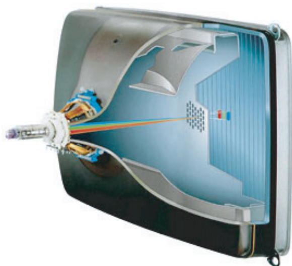
FIGURE 147 A cathode ray tube in older televisions: the first way – now obsolete – to produce changing colour images using electric signals. Television tubes emit an electron beam, deflect it, and generate light by electroluminescence on a coloured screen covered with patterned phosphors.
