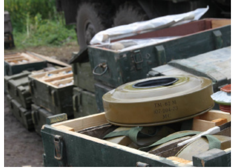
Photo 75 A TM-62M anti-vehicle landmine with MVZ-62 fuze, recovered from pro-Russian separatist forces.
