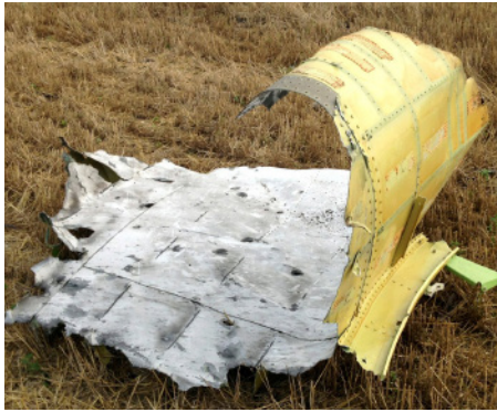
Photo 100 A piece of wreckage from MH17, showing damage consistent with a hit from a fragmenting missile warhead.
