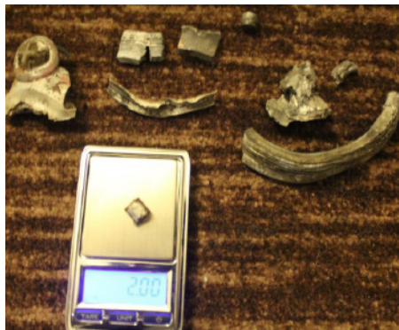
Photo 94 Remnants of a 9N210 HE-FRAG submunition identified by ARES for VICE News.
