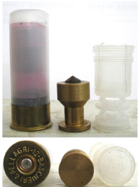
Photo 2 A reference image of the armour-piercing 'car stopper' 12 gauge cartridge, believed to be developed and produced by the Spetstekhnika design bureau in Kiev.
