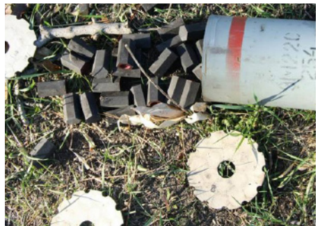
Photo 92 The remnants of a 9M22S rocket which failed to function. Located between the villages of Oleksandrivka and Chumaky, eastern Ukraine, November 2014. Photo credit: Mark Hiznay / Human Rights Watch.
