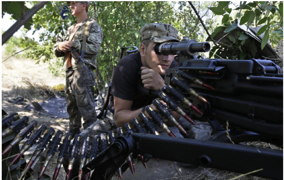
Photo 45 Pro-Russian rebels armed with an NSV heavy machine gun defend a position on the frontline near the village of Krasnodon, eastern Ukraine. Note the combination of BZT/BZT-44M armour piercing incendiary tracer (API-T) and MDZ high explosive incendiary (HEI) cartridges.
