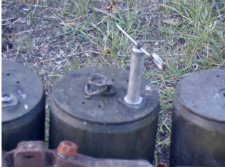
Photo 74 An OZM-72 bounding anti-personnel landmine, fitted with a MUV type pull fuze, and intended for use with a trip wire.
