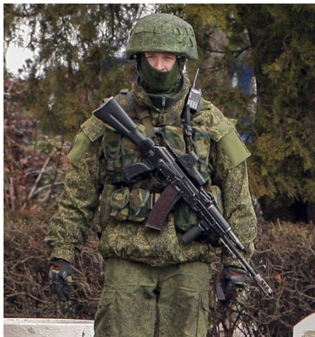
Photo 10 Unidentified uniformed combatant (presumed to be a Russian soldier) armed with an AK-74M rifle, Crimea, March 2014. Note EOTech type reflex sight, and Zenitco accessory rails, vertical foregrip, DTK-1 muzzle brake.
