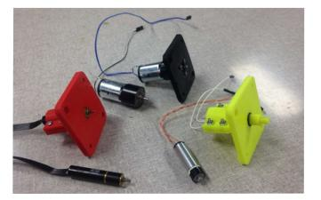
Fig. 3. Adapter plates for three different motors. (center) Face-mounted screws, (left) clamp for round motor housing only, and with (right) added shaft adapter .
