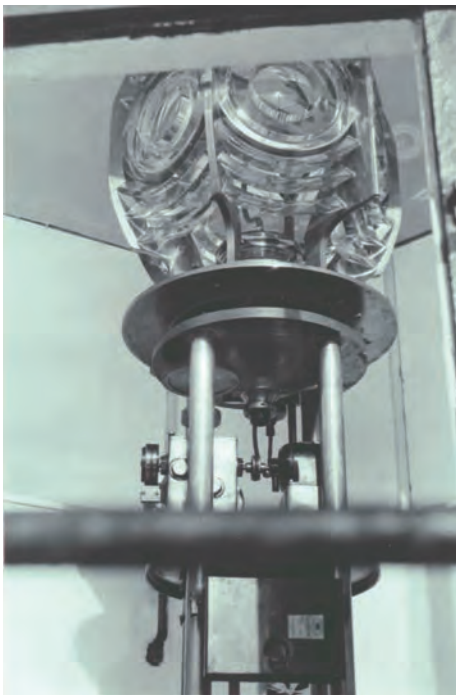
The Fresnel lens as it appeared when it was still in the lantern of Smith Island Lighthouse. The lens is now on display at the Museum of History and Industry in Seattle, Washington. (Don Skiff photo, Lighthouse Digest archives.)
