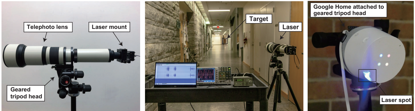
Fig. 1. Experimental setup for exploring attack range. (Top) Floor plan of the 110 m long corridor. (Left) Laser with telephoto lens mounted on geared tripod head for aiming. (Center) Laser aiming at the target across the 110 m corridor. (Right) Laser spot on the target device mounted on tripod.
