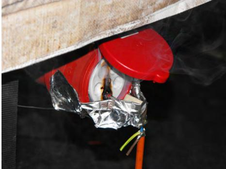
Figure 4 Localised damage to inner plastic core
