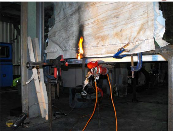
Figure 7 Ignition of curtain material following direct application of gas burner to webbing strap
