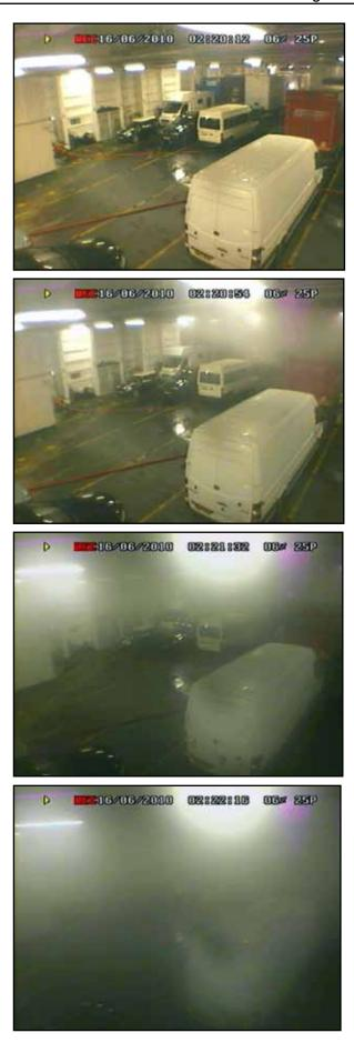
Cloud of steam from the upper vehicle deck as boundary cooling was started (CCTV timings are in UTC)
