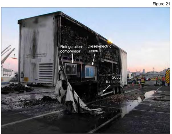
Diesel generator, refrigeration compressor and fuel tank
