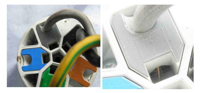
Figure 24 Conductor strands in connector
