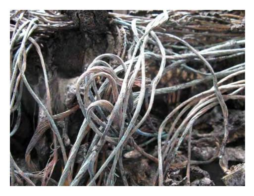
Figure 11 Fire damaged wiring
