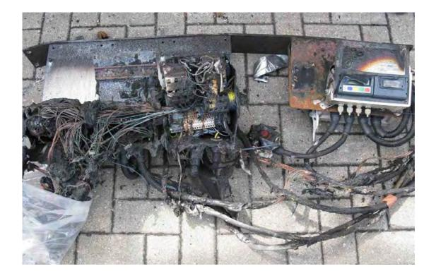
Figure 4 Control box assembly, fire damaged
