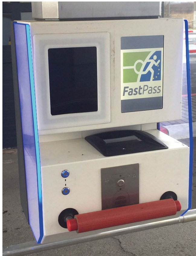
The travellers drove to the gate in a vehicle, at which point a unit with a facial recognition camera and a passport reader automatically moved next to an open window of the vehicle.
