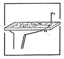
The spatial deformation of the front edge of the platforms as a result of Px = Py = Pz = 100 kiloponds (kilograms force) shall be a maximum of 1 mm (see drawing).
