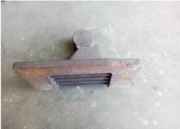
Fig.1 Shrinkage Defects in casting
